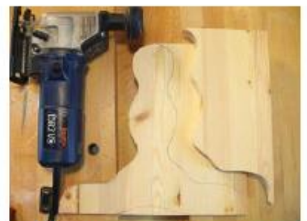
Pattern. Use the offcut from the first half of your side piece to mark the matching shape on the remaining three cuts.
