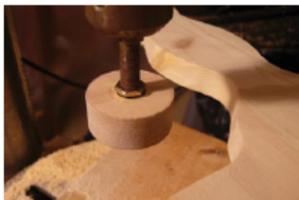
On the cheap. Glue a piece of sandpaper around a hole cutout, then mount it on a bolt with lock nuts – instant drum sander!
