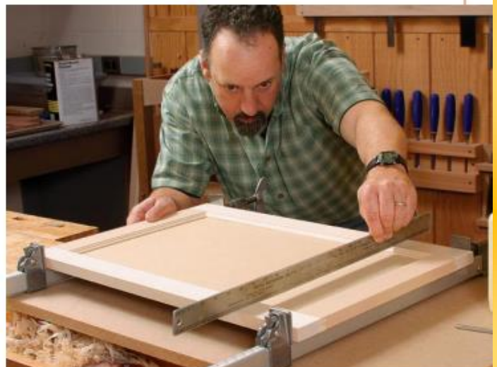
Check and clamp. Before tightening the clamps, use a straightedge to make sure the panel is flat in all directions. Adjust the clamps if necessary, and tighten.
