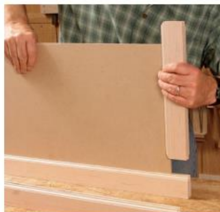
Attach the rails. After applying glue to the leading end of one rail, slide it down the panel edge and fit its stub tenon into place in the stile groove. Do the same with the second rail. Complete the assembly by gluing on the last stile.
