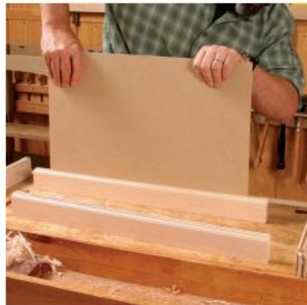
Placing the panel is key. Line up the panel precisely between the layout marks, and push it down to the groove bottom. This will keep the rest of the assembly square.
