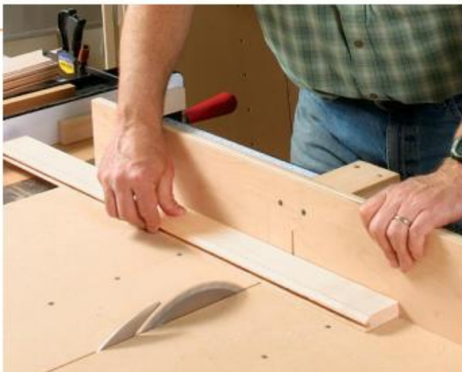
Cut all the stiles. Lead with the profiled edges to keep them free of chipout. A well-made crosscut sled keeps the cuts square.
