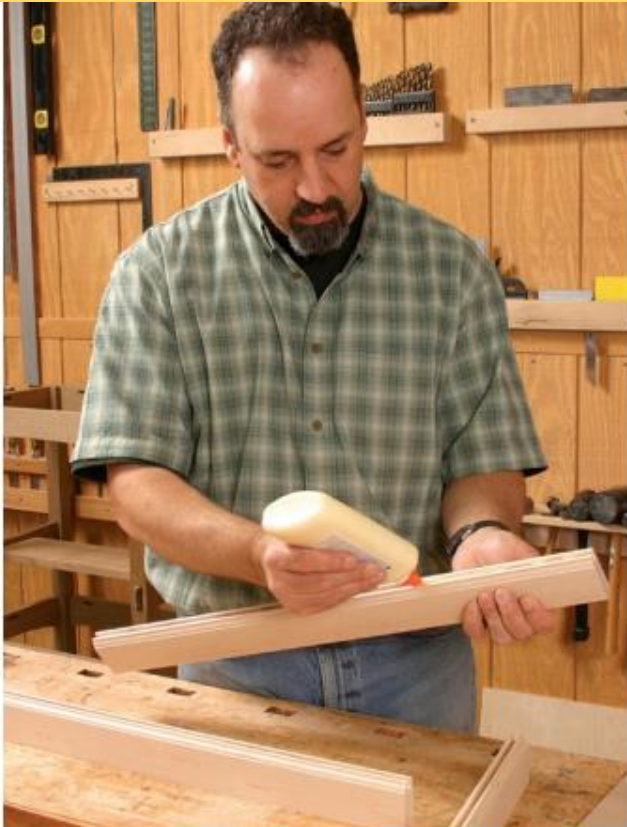
Mark and glue one stile. After marking the location of the panel on one of the stiles, apply glue inside the entire length of the stile's groove. The panel will be glued to the stiles only.
