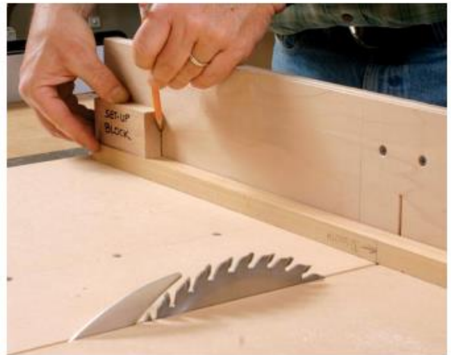
Use the block to set up the cut. With the story stick's door-width mark aligned with the sawblade, use the block to draw a line on the sled fence.
