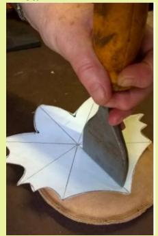
The next stage was to create creases along the leaf veins marked with the lines to each point of the leaf. H&R once again improvised for a creasing tool by rounding off a masonry chisel and using a circular leather sandbag. The sandbag supports the copper, but allows some
