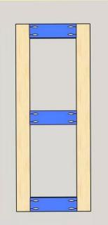
The holes need to be drilled along the grain of the wood whenever possible, as drilling across the grain will result in a much weaker joint.
