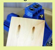
The use of pocket holes makes the aligning of the two pieces of timber really easy, just clamp the joint before driving in the screws.
