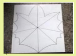
So, the leaf design was to be based on a maple leaf from the garden, with a card template used to draw on the copper sheet, 0.5mm thick. The fold ines all met roughly in
