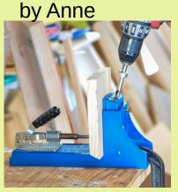
When attaching two pieces of wood, the Kreg jig enables you to drill angled holes into one of the
