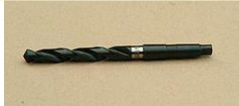
Twist drill bit with Morse taper shank
