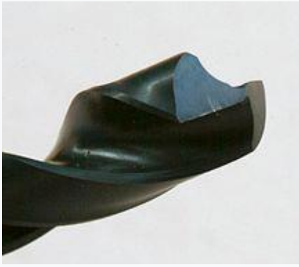
Twist drill bit cutting edges
