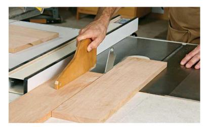
Ripping is a term used to define cutting a wooden plank across its length. Such a cut tends to be long and can be done using various means like using a free hand, using a rip fence or a circular saw. In most cases, Ripping is done on a table saw. If you don't do it the right way, there are chances that you may end up wasting a huge chunk of your wood.
