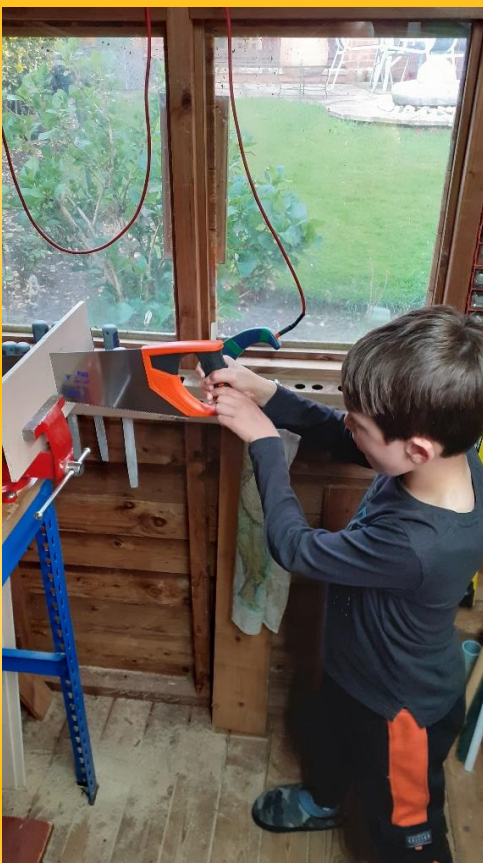
Pete's first cross-halving joint since school woodwork lessons Don't want any splinters – Tongue poking out aids concentration
